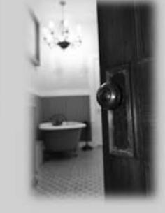
The hardware: knobs and pulls were cleaned (boiled, to be exact) repaired and reattached. Light fixtures in the Parlor, dining room and blassy and many others were re-wired and restored. Where original light fixtures had been lost, or additional lighting was needed, period light fixtures were acquired and re-wired.
